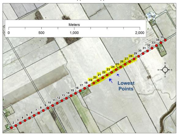
may be underwater during a 1:100 year flood event to a maximum depth elevation of 0.3 metres. The cost estimate is approximately \$200,000 for interim improvements to this road profile, including culverts and delineators.
