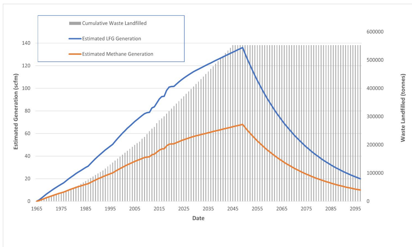
Figure B4-1: Estimated Landfill Gas and Methane Generation Rates from LandGEM Model
